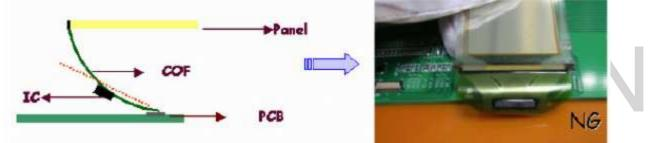
12.6 Use both thumbs to insert COF into the connector when assembling the panel. See the photo on the far right below for correct insertion of the film into the connector (one-handed insertion exerts uneven force on the film and could cause its breakage, photo on the left)
